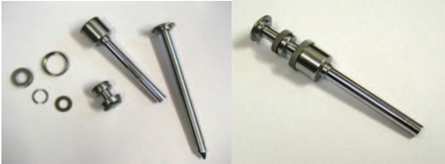
Fig. 7. To the left, the separate parts of a trocar. To the right, a fully assembled trocar.
