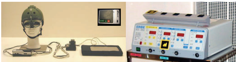
Fig. 5. To the right, the helmet-mounted Augmented Reality System. To the left, the electro-surgical generator prepared with markers for the tracking.
