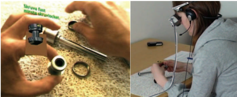
Fig. 8a) The participant's view in the HMD. b) A participant wearing the head mounted display and using the headphones and voice interaction to follow the AR instructions.
